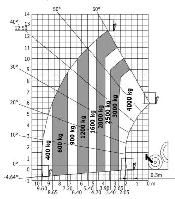
Machine on lowered stabilisers with forks Metric
